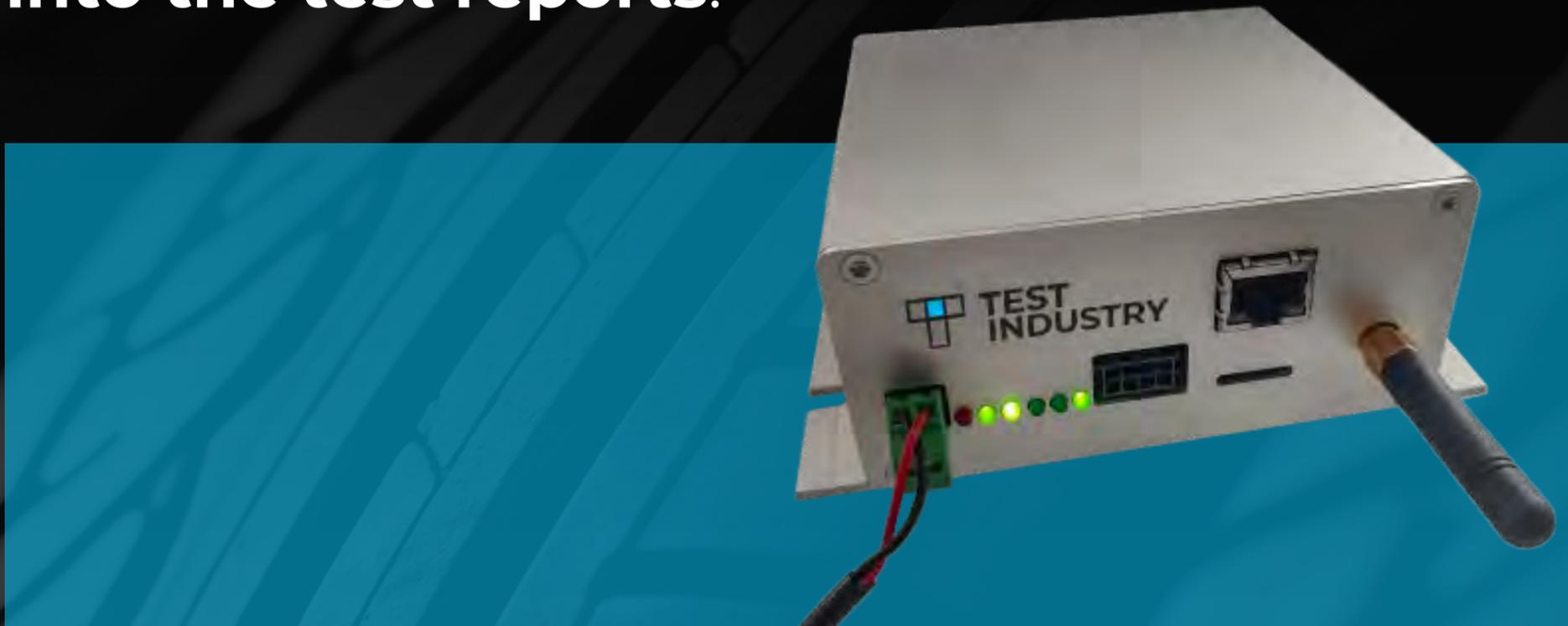
The system is provided with **Ethernet** and **RS485** interfaces, allowing easy integration into the measuring environment.
